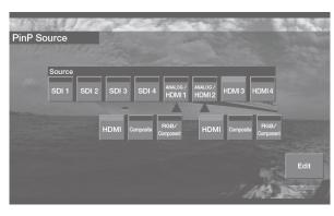
Touch a selection from <SDI 1>-<HDMI 4> to select the connector where the video to composite is input.
